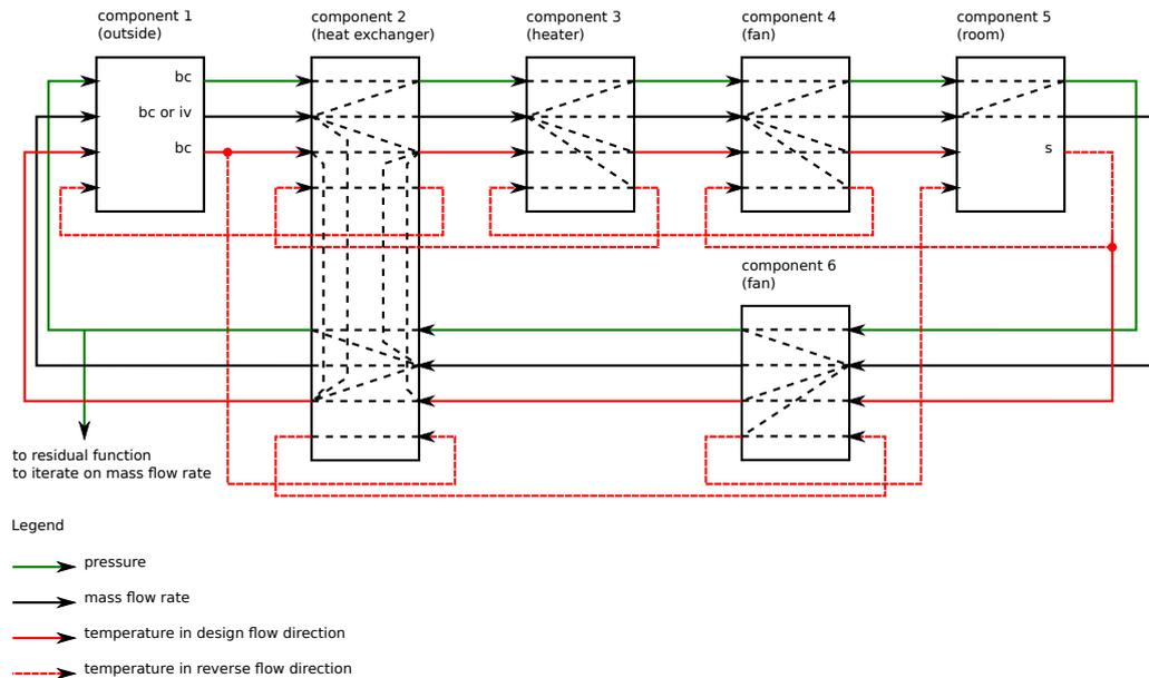
**Figure 10.** FMUs connected in a loop with a heat exchanger between the outside air intake and the exhaust air.
