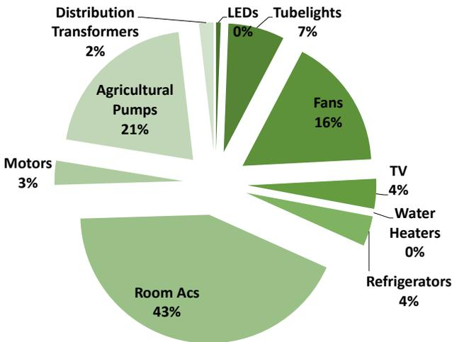
Figure 4: Breakdown of the peak load reduction in the Efficient Future scenario in 2030 (total reduction = 71GW)
