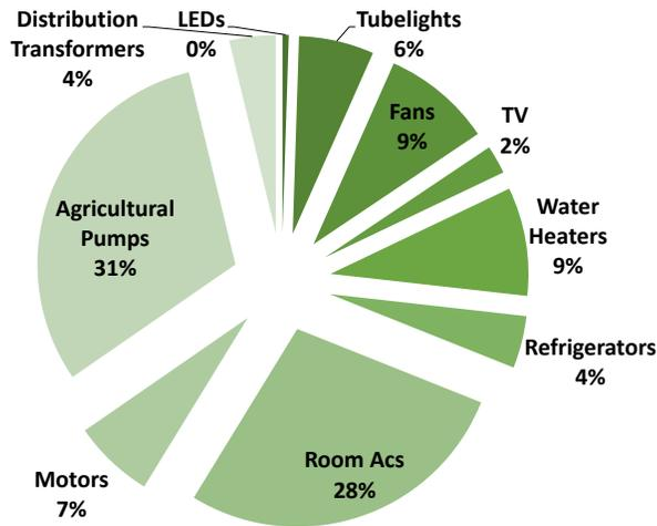
Figure 3: Breakdown of the total energy saving in the Efficient Future scenario in 2030 (total saving = 301 TWh/yr)
