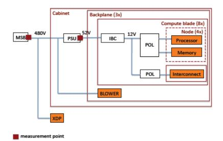
Fig. 2. Power monitoring capabilities for Jaguar
