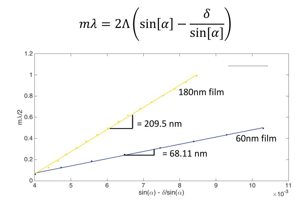
Correlation length overestimates film thickness compared to ellipsometry, but has the advantage of being in-situ
