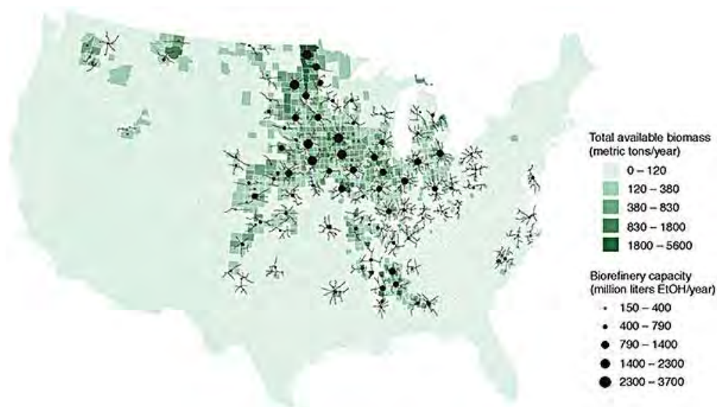
U.S. national cellulosic biofuels scenario including biomass production by county, simulated biorefinery locations and optimal rail paths for feedstocks.
