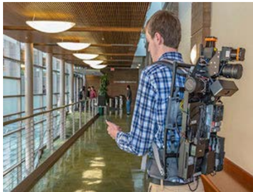
The Rapid Building Energy Modeler (RAPMOD) Backpack
