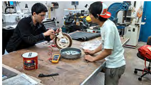
Jarrett Kodani and Kok Lim from the University of Hawaii disassemble a pancake-style 3-phase washer motor and measure its physical and electrical parameters for benchmarking.
