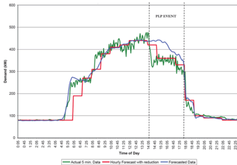
Performance of Contra Costa County office building in non-spinning reserves tests led by Berkeley Lab researchers.
