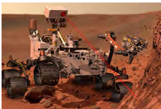
Artist's concept of rover Curiosity with LIBS technology firing a beam of infrared light at Martian rock for spectroscopic analysis. (Image courtesy of NASA)
