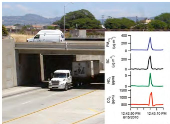
Figure 1. The mobile laboratory and pollutants measured in the exhaust of one truck. Note the air sampling inlet positioned above the vertical exhaust stack of the diesel truck driving toward the Port of Oakland.
