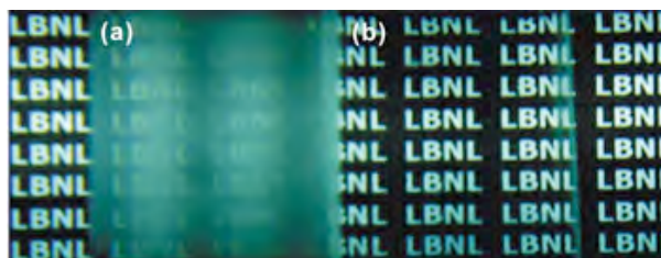
Figure 1. Nanostructured antifogging coatings have been applied to the right side (b) of the surface, which remains clear, while the untreated left side (a) forms condensation.
