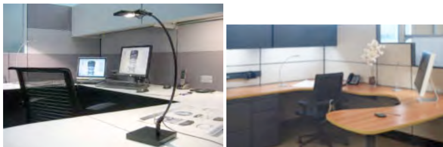
Figure 2. Modern hybrid lighting combines fluorescents with LEDs to deliver pleasing ambient light and strong targeted light for tasks.
