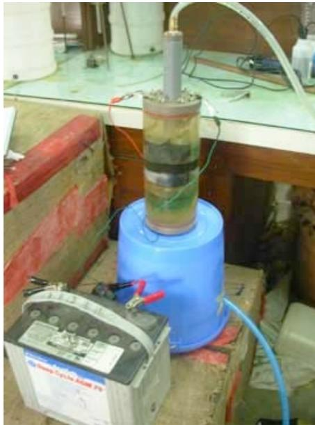
A small-scale ECAR prototype device operated from a 12-volt car battery at the Bangladesh University of Engineering and Technology (BUET), Dhaka, Bangladesh (July 2008).
