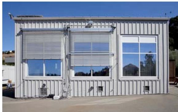
Berkeley Lab's Advanced Windows Test Facility is an example of an existing test bed that allows researchers to install prototypes or existing products and measure their performance over time, and under changing conditions.
