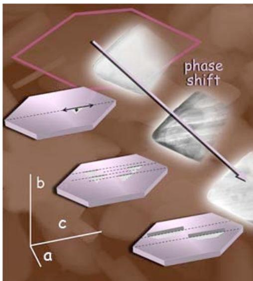
As lithium ions move out of a hexagonal lithium iron phosphate crystal, the material undergoes a phase shift to iron phosphate. Since ions flow only in the b direction, the ideal particle shape is a plate of lithium iron phosphate as thin as possible.
