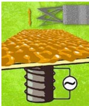
Current-sensing atomic force microscopy is used to measure both the conductance and the surface topography of electrode materials, with resolution at micrometer and nanometer scales.
