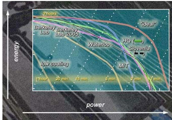
The performance of batteries developed by groups at Berkeley Lab, MIT, Hydro Quebec, and in Slovenia is compared. All batteries use similar lithium compounds but are engineered differently. The red curve, based on a model by Venkat Srinivasan, shows the theoretical maximum performance of electrodes using compounds such as lithium iron phosphate with graphite.
