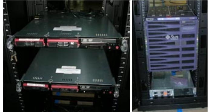
Figure 2. Servers modified to accept 380V DC
