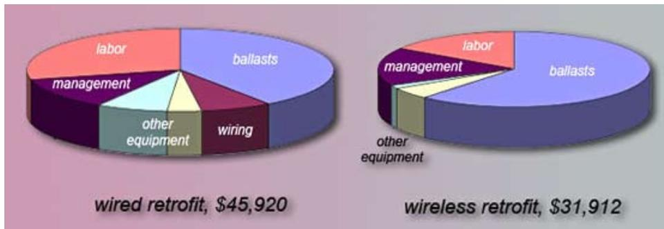
*A wireless network installation is estimated to cost 30 percent less than a wired network installation. Much of the savings is in labor (and there is no cost for wire).*
