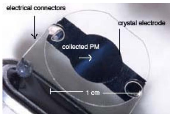
**Figure 1.** The blue streak shows a track of particles deposited on the quartz crystal microbalance of a Berkeley Lab prototype. A thermophoretic heater located above the crystal substrate precipitates particulate matter from the air onto the microbalance.
