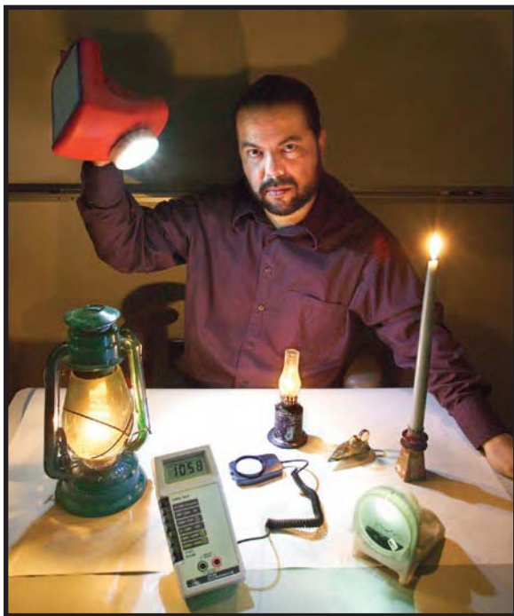
Figure 1. Evan Mills holds a prototype white light-emitting diode (WLED) made by a company called Ignite Innovations. This lamp, which grew out of a Stanford-led effort involving several Silicon Valley companies, Berkeley Lab, and others, features a one watt WLED, solar panel and rechargeable AA batteries. (Photo by Roy Kalischmidt)
