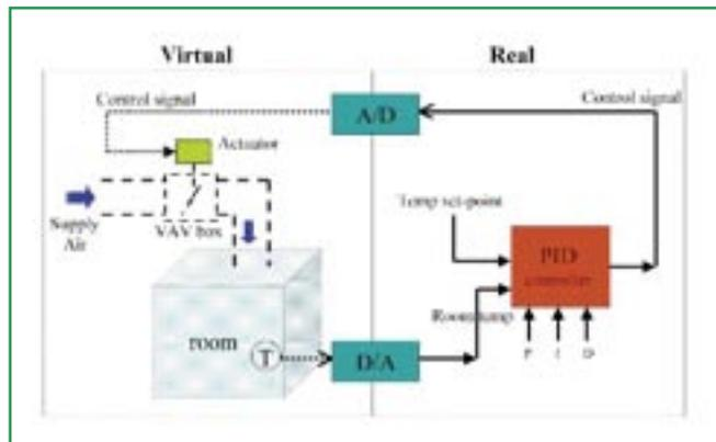
Figure 3. VAV control simulator example: hybrid software-hardware configuration
