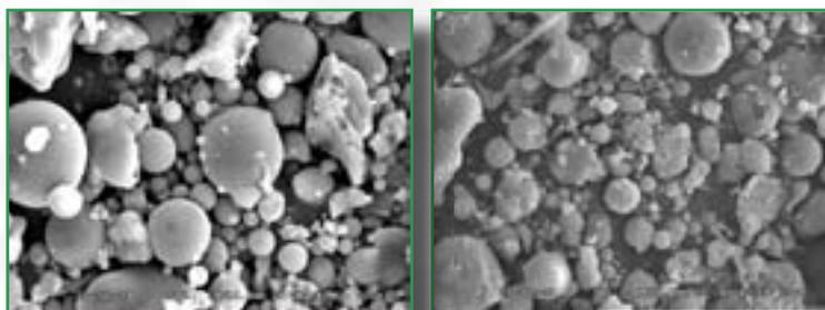
**Figure 1.** Bottom ash before (left) and after coating with ferric oxide
