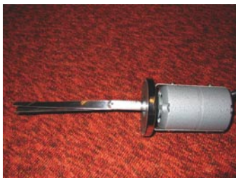
Figure 1. The whip injector; note the small, light weight CO 2 cylinder
