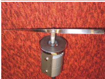
Figure 2. The mixing fan, with blades folded for insertion in the duct (top) and with blades unfolded
