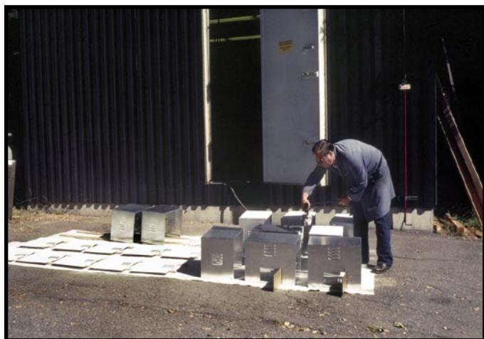
Figure 5. Dick Schmidt inspects carbon aerosol sampling equipment
