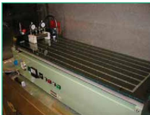
Figure 2. Electrode casting device.
