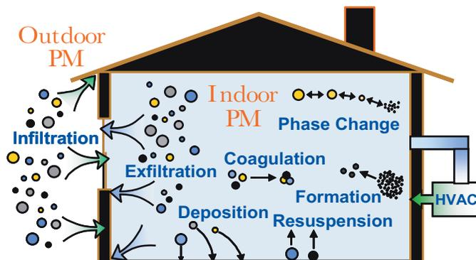
Figure 2. Schematic of the Clovis, CA research house showing the important processes that affect the indoor concentration of outdoor PM<sub>2.5</sub>.
