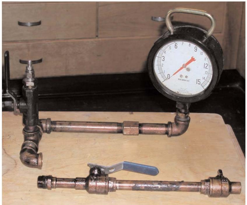
Figure. Oil-sampling device developed for heavy oil tank emissions test.
