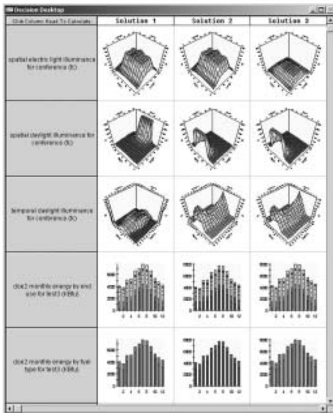
For energy analyses, BDA supplies DOE2.1E with hourly weather information along with a description of the building and its HVAC equipment and occupancy patterns. The energy-related performance parameters that can be computed include annual and monthly energy-use values broken down by end use and by fuel type. BDA 3.0 also supports DOE2.1E parametric evaluations of energy requirements by end use as a function of window-to-wall ratio, allowing quick and easy optimization of window size.
