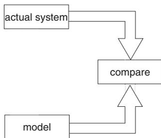
Figure 1. A model-based fault detection scheme
