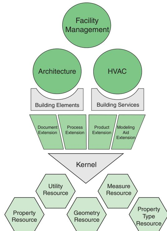
Figure. Architecture of the IFC object data model.
