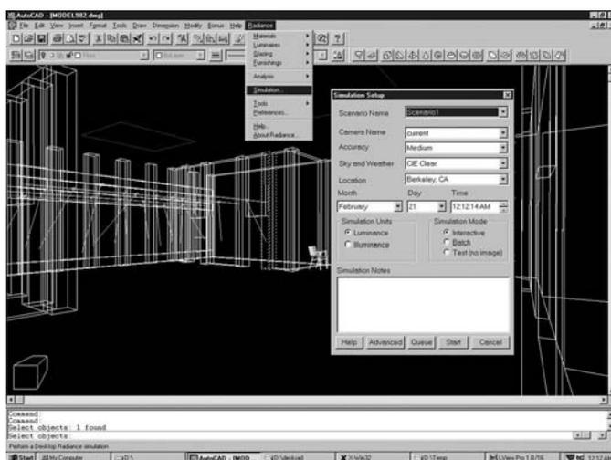
*Users can control the Radiance algorithms through a graphical user interface accessible from within AutoCAD.*
