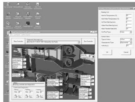
Figure 2: Screen shot showing an implementation for a dual-duct air-handler system
