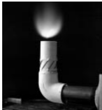
A burner built from inexpensive plastic pipe shows the adaptability of the low-swirl burner (left). The ring stabilizer keeps the flame steady (right).
