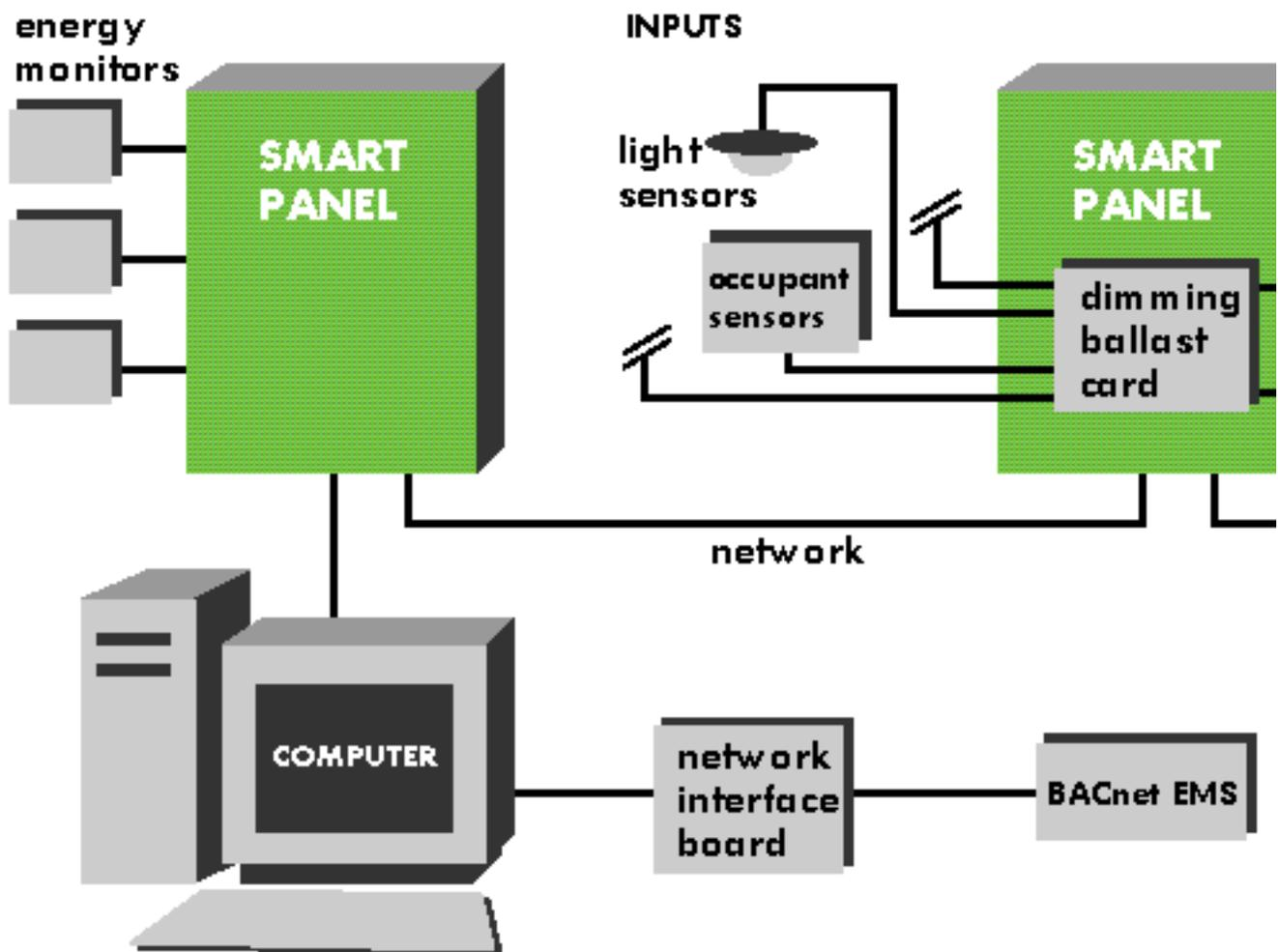
Figure 3: Occupant sensors, photocells, manual switches, and energy monitors are all connected to 40 "smart panels" distributed strategically throughout the three-floor testbed. All the smart panels are interconnected and communicate over a simple twisted pair of wires.
